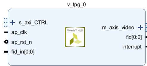
Figure 22. Video Test Pattern Generator
