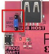
Figure 66. Program jumper setting
