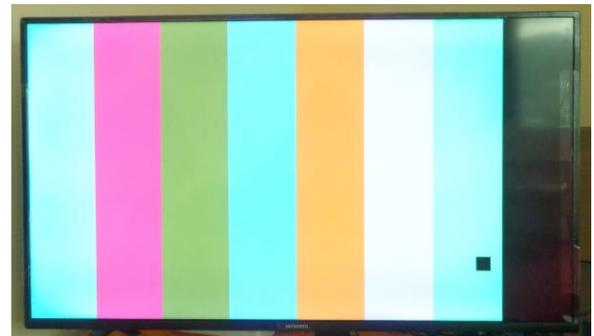
Figure 84. Output obtained after converting RGB into YUV444
