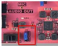
Figure 67. Power jumper setting
